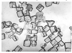
Fig.2 Micrograph of AgBr microcrystals of 2<sup>nd</sup> type sampled at 10 min after start of etching in 1% Na<sub>2</sub>S<sub>2</sub>O<sub>3</sub> solution. Magnification 10000×.
