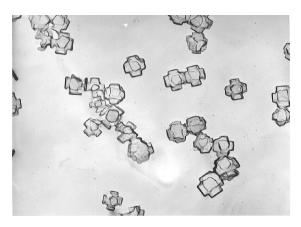
Fig.1 Micrograph of AgBr microcrystals of 1<sup>st</sup> type sampled at 10 min after start of etching in 1% Na<sub>2</sub>S<sub>2</sub>O<sub>3</sub> solution. Magnification 10000×.
